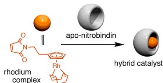
Figure 2. Preparation of a hybrid biocatalyst involving a rhodium complex via a covalent linkage between maleimide and a thiol group of Cys96 in the cavity of nitrobindin.
